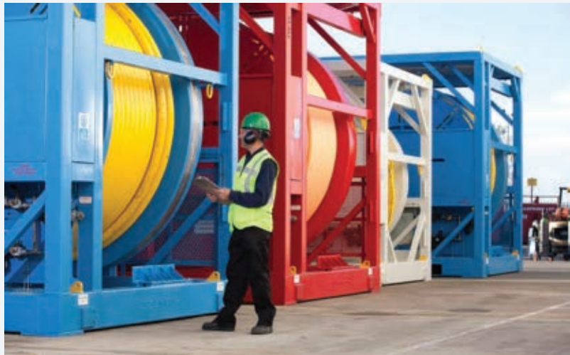
Comprehensive pre-deployment inspection and testing ensured successful installation of the IWOC umbilicals for the Jack/St. Malo project.
